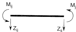
Figure B.5 End moments and vertical end forces on a beam member
