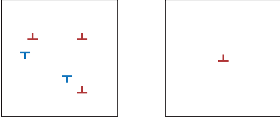
Fig. 2.2 Coarse graining applied on strongly different dislocation arrangement can lead to the same signed dislocation densities at some points. This two configurations gives the same signed dislocation density \kappa at the center using a window function represented by the box.
